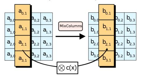
1 means don't change the value, 2 means left shift by one bit, and 3 means left shift by one bit and XOR with the original value
